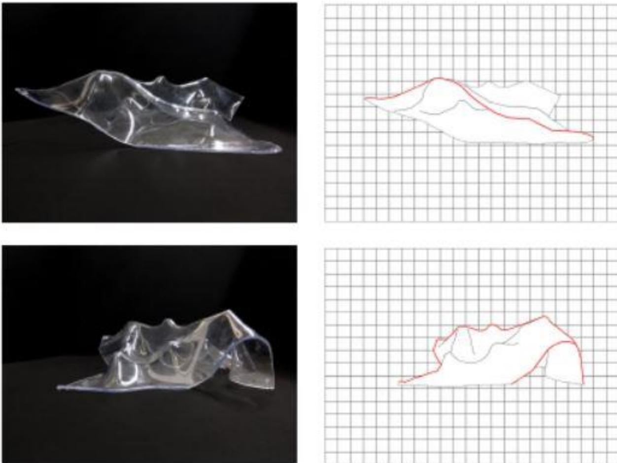
Figure 11(b) Acrylic sheet placed on points with different heights subjected to heat linearly.
