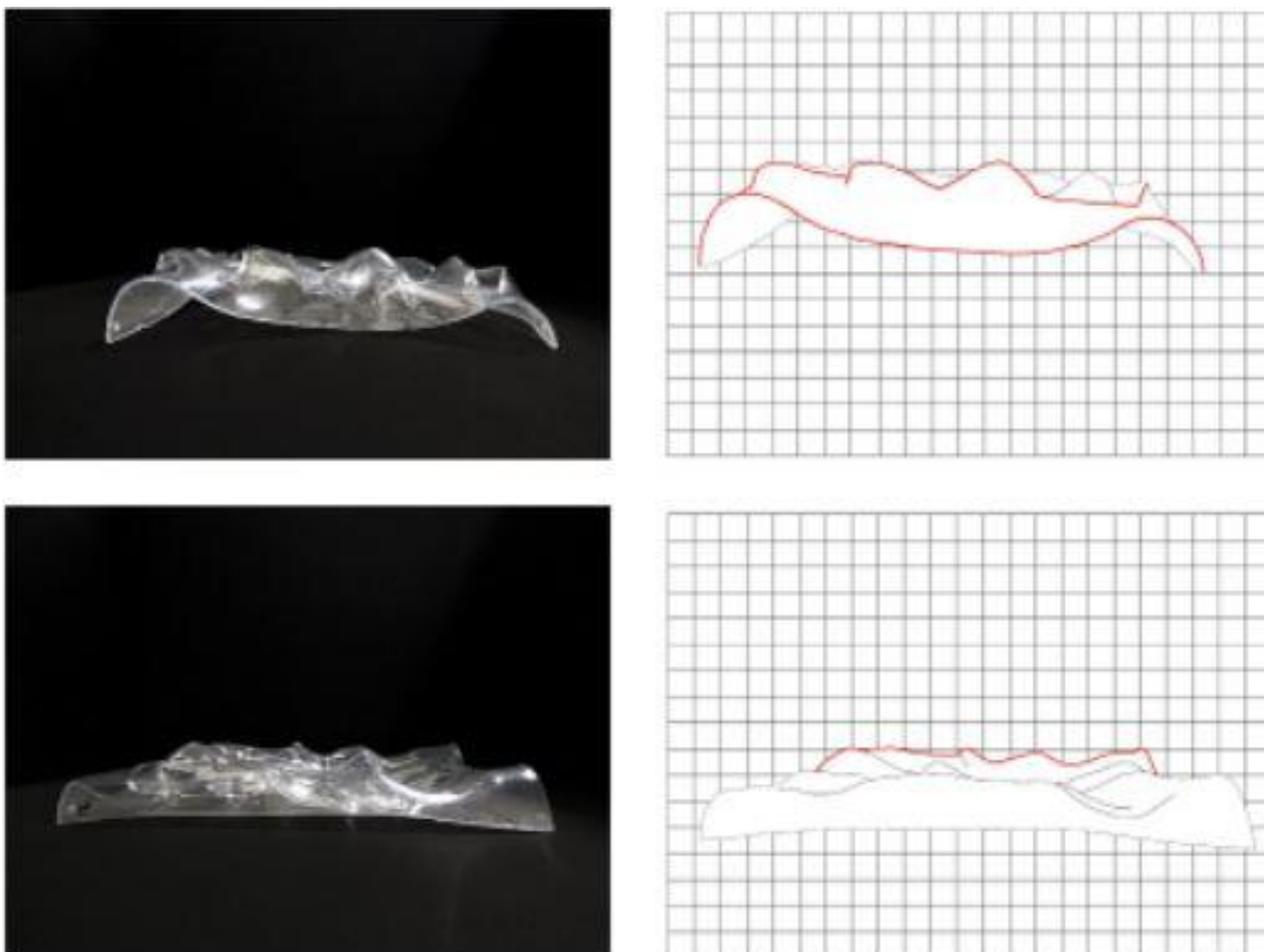
Figure 10(b) Acrylic sheet placed on points subjected to heat linearly.
