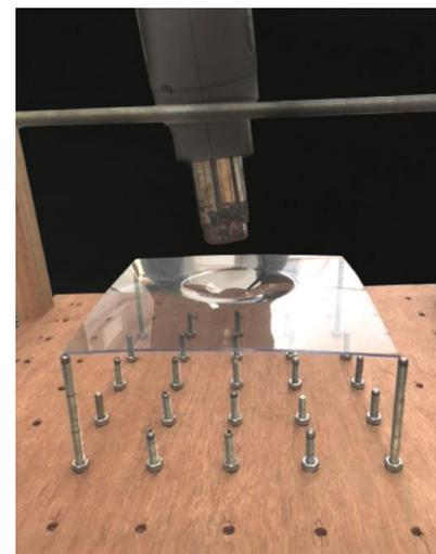
Figure 4, Acrylic sheet placed on points subjected to heat centrally.
