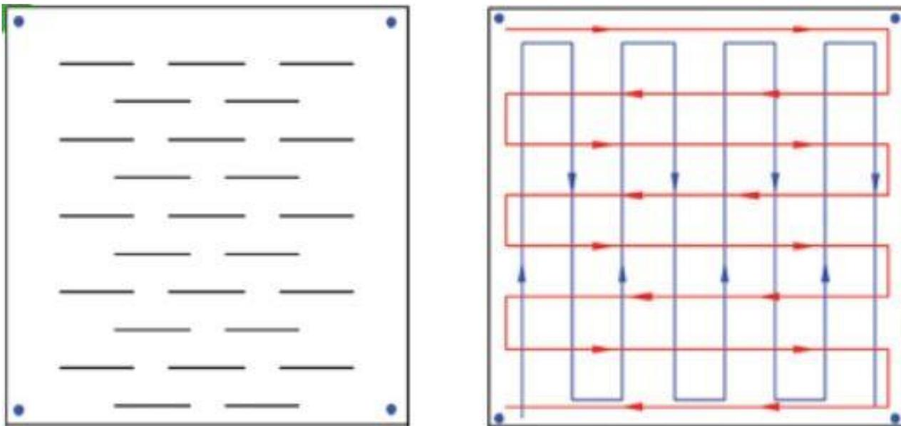
Figure 10(a) Acrylic sheet placed on points subjected to heat linearly.
