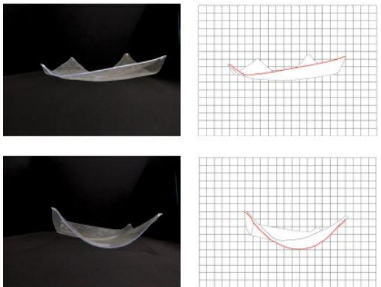
Figure 7, Acrylic sheet placed on points subjected to heat diagonally.
